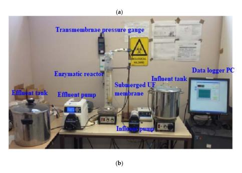
**Figure 2.** A schematic diagram (a) and a photography of laboratory scale enzymatic membrane reactor (b).
