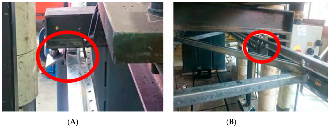
Figure 8. Crippling of load points: (A) Typical crippling at flanges; (B) Specific crippling reinforcement.
