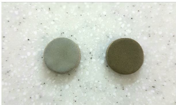
Fig. 12 – Appearance of GC0.29 after immersion in HCl (left) and NaOH (right) solutions for 6 h.
