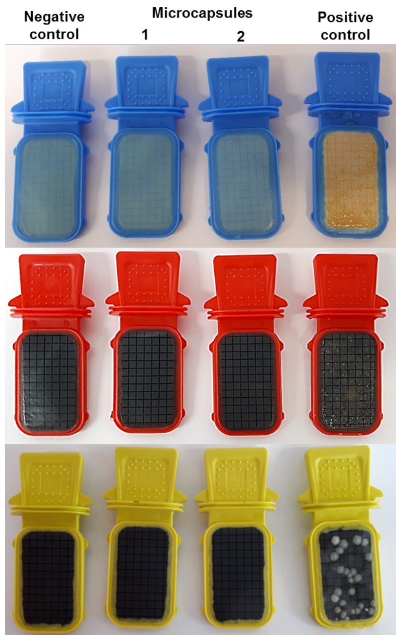
Figure S4. Photographs of sterility testers analysing the presence of microorganisms, comparing a negative control (sterile water), two different batches of microcapsules with AuNPs (microcapsules 1 and 2) and a positive control of contamination (ground sample). Coliform organisms were tested using the Coli-Count™ Sampler (blue), aerobic bacteria using HPC Total Count Sampler (red) and yeast or moulds employing the Yeast and Mould Sampler (yellow).
