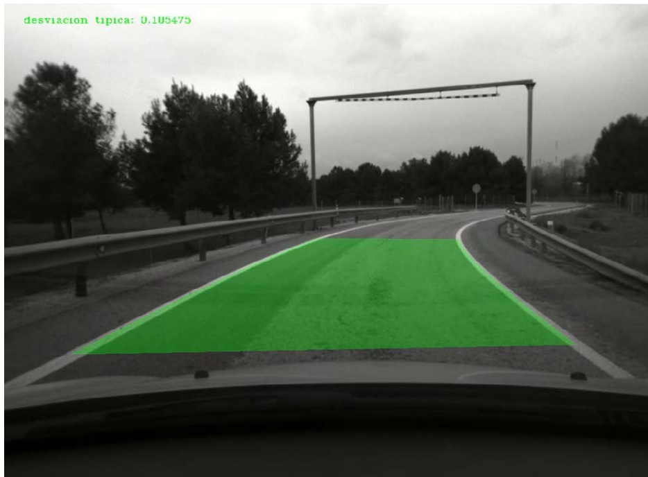
(A) The road corridor is shaded green as the detection is considered valid ( \sigma_w < th_{\sigma_w} )
