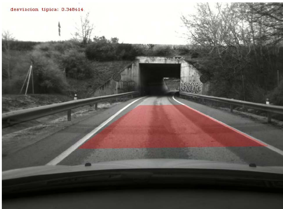
(B) The road corridor is shaded red as the detection is considered invalid ( \sigma_w > th_{\sigma_w} )
