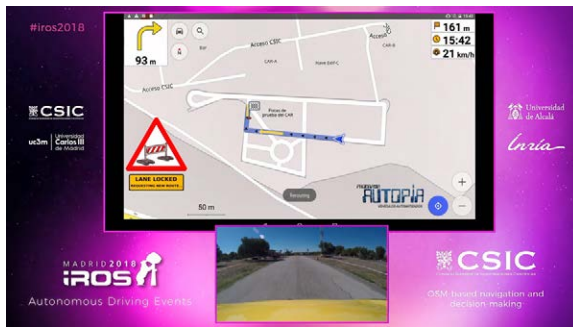
(B) Re-routing due to road blockage. Blocking obstacle detected and re-routing request
