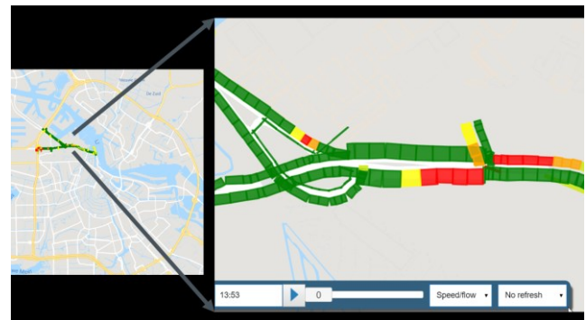
Fig. 17: Framework with network and traffic model for short term prediction.
