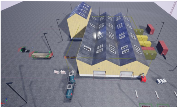
Fig. 13: Simulated parking station environment for back maneuvering assist developed with Unreal Engine.
