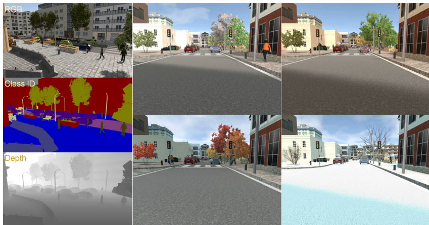
Figure 10.3.5 SYNTHIA: RGB image, ground truth for Class ID and depth; images acquired from the same camera location at different seasons.
