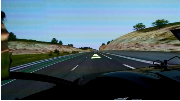
Figure 8.9 Example of an augmented reality evaluation study for an automated driving prototype (carried out at CTAG's driving simulator).
