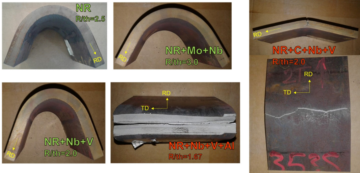
Figure 122. Examples of 12mm HT-TMCP bend samples.
