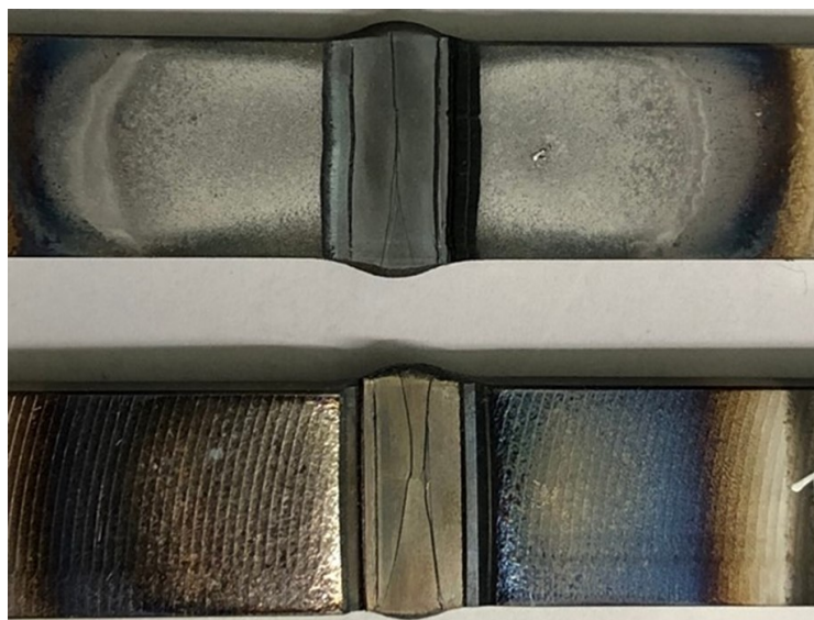
Figure 65. LT-TMCP-3mm HDS-V40 samples with imprints from the deformation stamps broken during the deformation at 350 °C.
