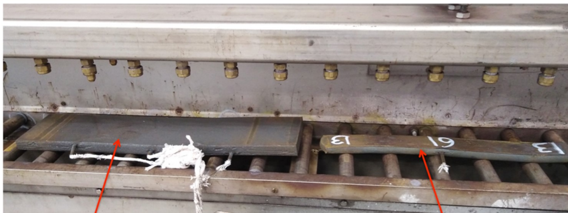
Figure 137. Image illustrating the width differences between calibration sample and actual sample used during the TMCP simulations.
