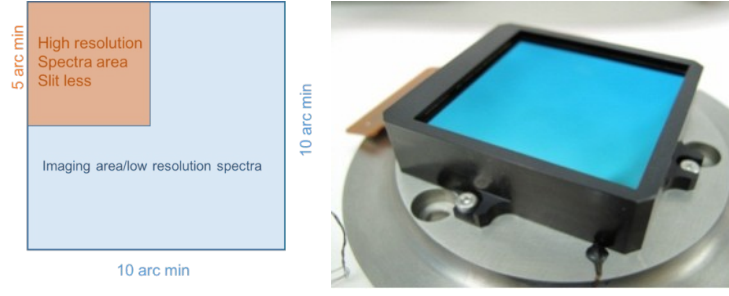
Figure 39: Left : the IRT focal plane division. The blue area ( 10 \times 10 arcmin) is used for imaging and low resolution spectra. The orange area ( 5 \times 5 arcmin) is used for high-resolution slit-less spectra. The size of the high-resolution spectral area is limited by the satellite pointing capabilities. Right : Teledyne Hawaii 2RG detector at ESA Payload Technology Validation section during the tests for the NISP instrument on board the EUCLID mission (Credits ESA).
