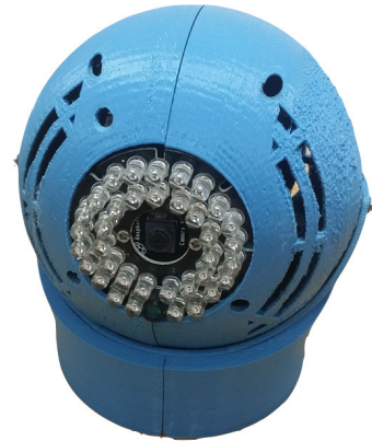
FIGURE 1. Fall detection system prototype.
