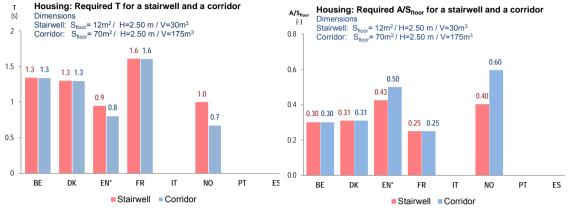
\* Method A acc. Approved Document E. Resistance to sound has been applied. The reverberation time and A/S<sub>floor</sub> were calculated for a minimum  $\alpha_w$  of a class D absorber.
