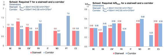
\* Method A acc. Approved Document E. Resistance to sound has been applied. The reverberation time and A/S<sub>floor</sub> were calculated for a minimum  $\alpha_w$  of a class D absorber.
