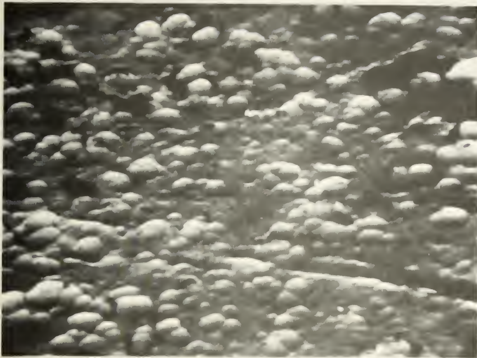
Figure 14. One micron silicon coating over polished 2024 aluminum before irradiation.
