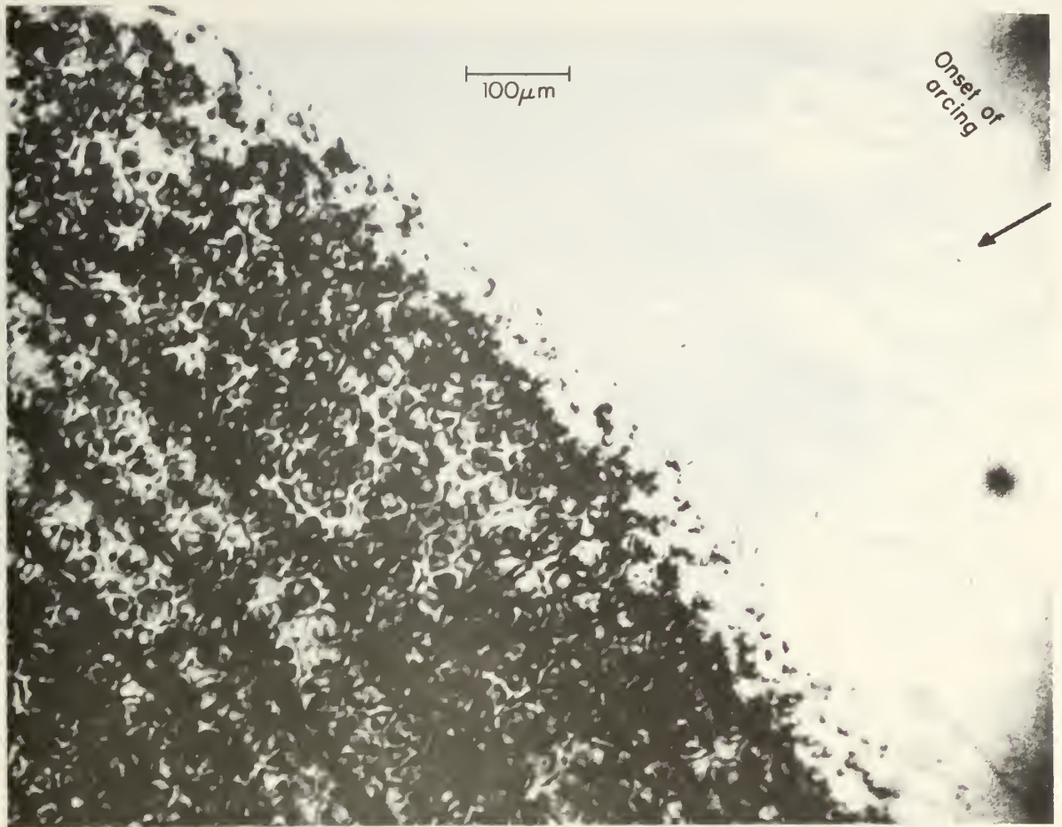
Figure 10. Laser-produced arc pattern near edge of laser illuminated area. Arrows show onset of arcing in ring pattern.
