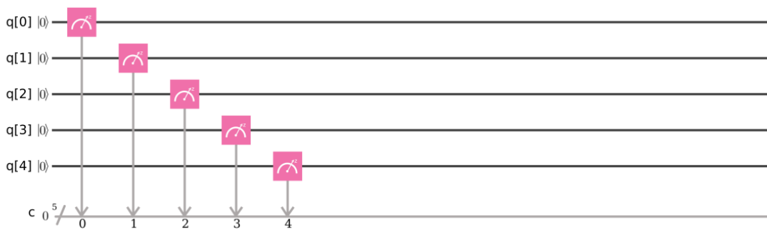
Figure 3.9. Experiment 3.1: Measuring the initial state.
