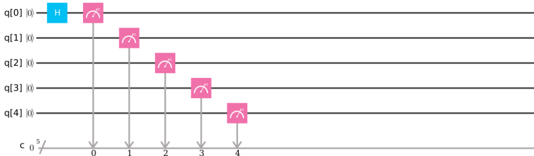
Figure 3.15. Experiment 3.4: q_0 into superposition with five measurements.
