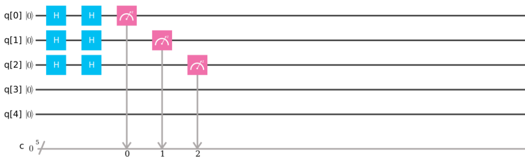
Figure 4.3. Experiment 4.1: Deutsch-Jozsa constant equation example. Source: [10].
