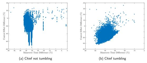
Figure 6.18. Comparison of NMPC and MT-OCP maneuver time and control effort results for position (NMC velocity, aligned attitude) subspace.
