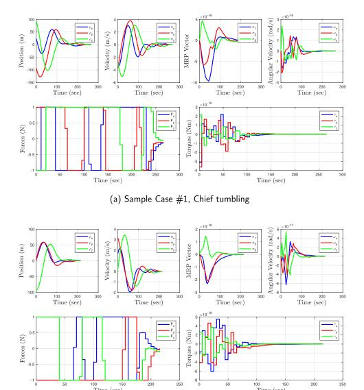
Figure 6.20. Sample NMPC closed-loop cases from position (NMC velocity, aligned attitude) with tumbling chief.
