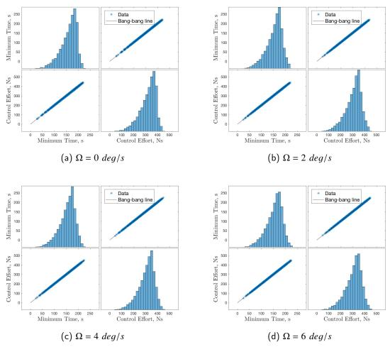
Figure 4.17. Minimum time and control effort histograms and correlation for position (NMC velocity) subspace.
