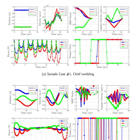
Figure 5.20. Sample cases from attitude (zero angular velocity, rendezvous position) subspace with tumbling chief.
