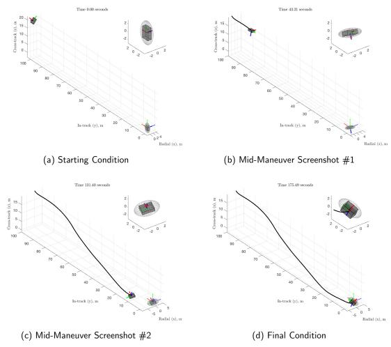
Figure 7.51. Case 7–relative trajectory for minimum time maneuver.
