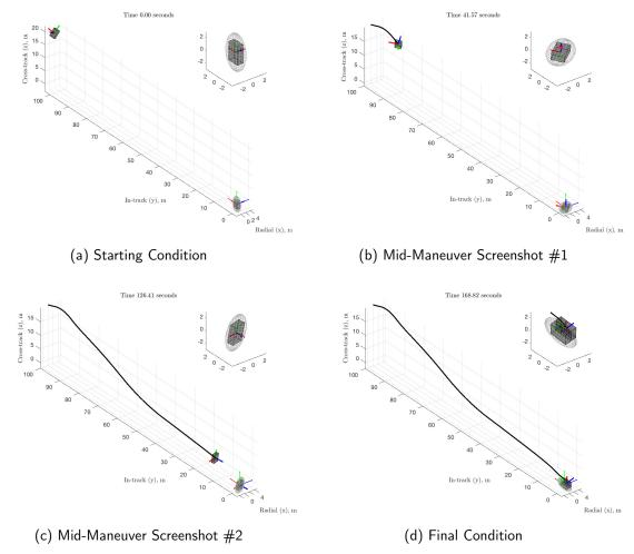
Figure 7.43. Case 6-relative trajectory for minimum time maneuver.
