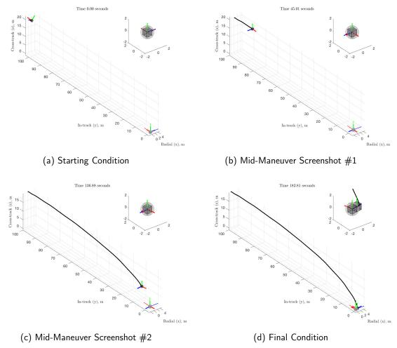
Figure 7.11. Case 2–relative trajectory for minimum time maneuver.
