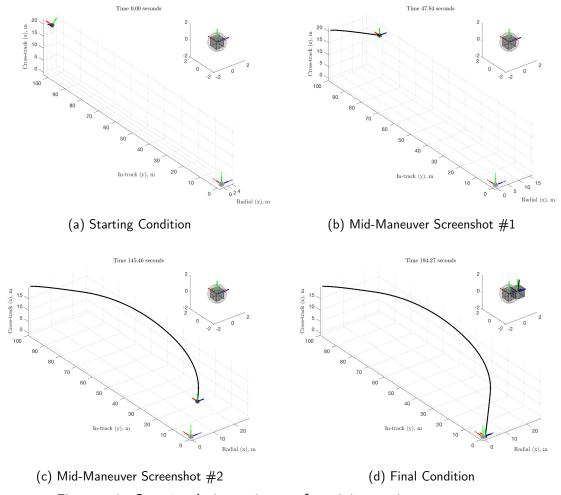
Figure 7.3. Case 1-relative trajectory for minimum time maneuver.
