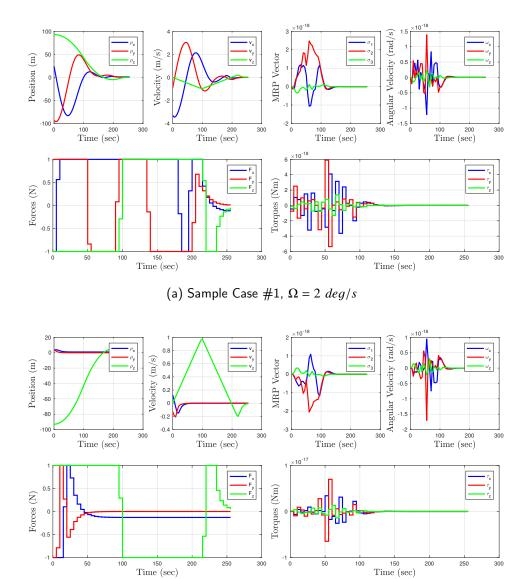
Figure 6.6. Sample NMPC closed-loop cases from position (NMC velocity, aligned attitude) for  $\Omega=2\ deg/s$ .
