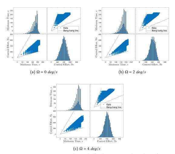
Figure 5.3. Minimum time and control effort histograms and correlation for position (NMC velocity, aligned attitude) subspace.
