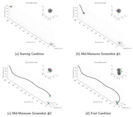
Figure 7.19. Case 3–relative trajectory for minimum time maneuver.
