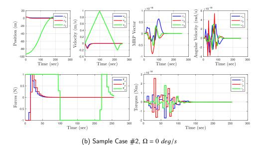
Figure 6.5. Sample NMPC closed-loop cases from position (NMC velocity, aligned attitude) for  $\Omega = 0 \ deg/s$ .
