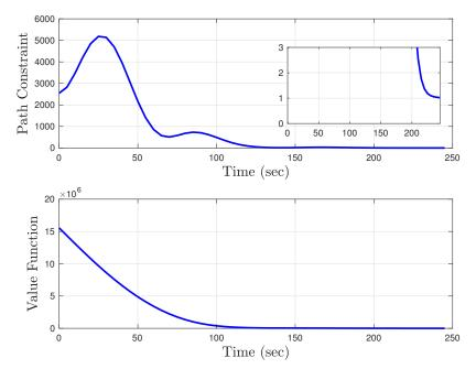
Figure 7.58. Case 7–verification of KOZ constraint satisfaction and time history of NMPC value function.
