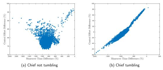
Figure 6.24. Comparison of NMPC and MT-OCP maneuver time and control effort results, for attitude (zero angular velocity, rendezvous position) subspace.
