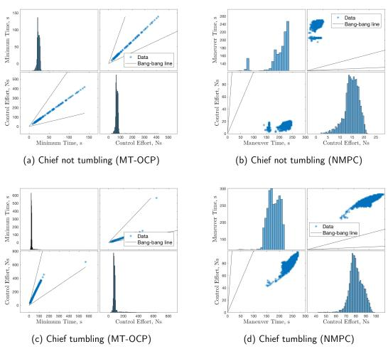
Figure 6.23. NMPC maneuver time and control effort histograms and correlation for attitude (zero angular velocity, rendezvous position) subspace.
