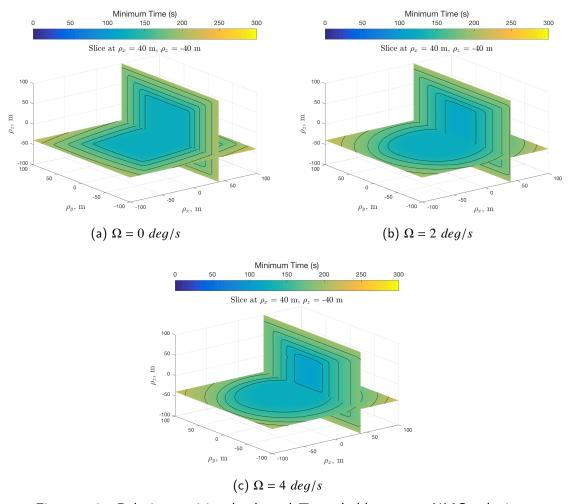
Figure 5.2. Relative position backward T-reachable sets at NMC velocity, aligned attitude, and zero angular velocity at different chief rotation rates, sliced at  $\rho_x = 40~m$  and  $\rho_z = -40~m$ ; color bar indicates minimum time values corresponding to the contours.
