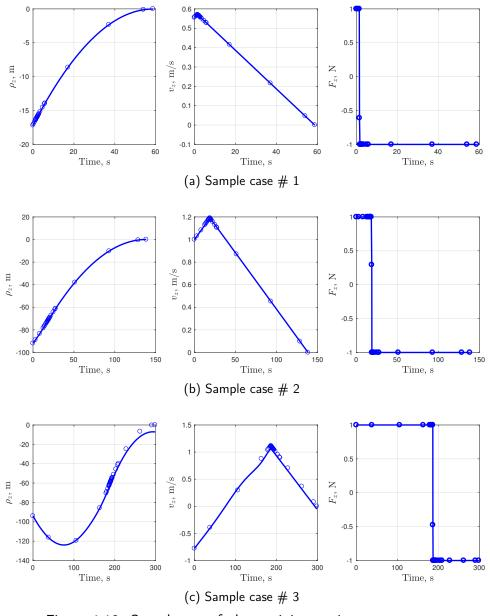
Figure 4.10. Sample out-of-plane minimum time maneuvers.
