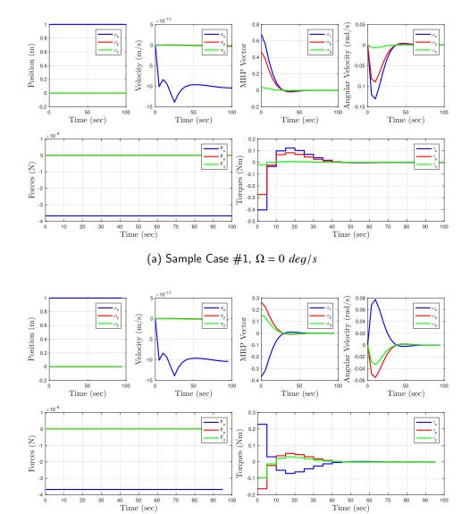
Figure 6.12. Sample NMPC closed-loop cases from attitude (zero angular velocity, rendezvous position) for  $\Omega = 0 \ deg/s$ .
