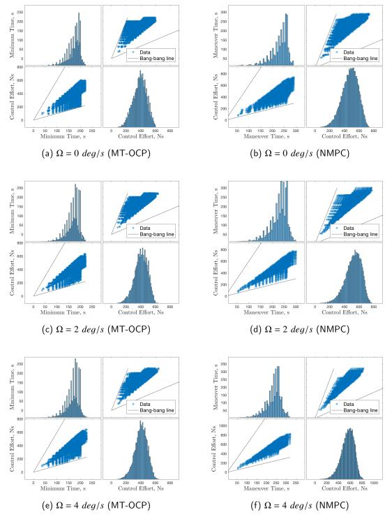
Figure 6.3. NMPC maneuver time and control effort histograms and correlation for position (NMC velocity, aligned attitude) subspace.
