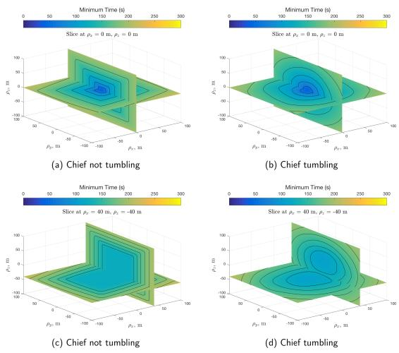
Figure 5.13. Relative position backward T-reachable sets at NMC velocity, aligned attitude, and zero angular velocity with tumbling chief, sliced at  $\rho_x = 0$  m and  $\rho_z = 0$  m and  $\rho_z = 40$  m and  $\rho_z = -40$  m; color bar indicates minimum time values corresponding to the contours.
