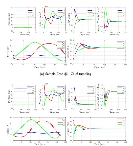
Figure 6.26. Sample NMPC closed-loop cases from attitude (zero angular velocity, rendezvous position) with tumbling chief.
