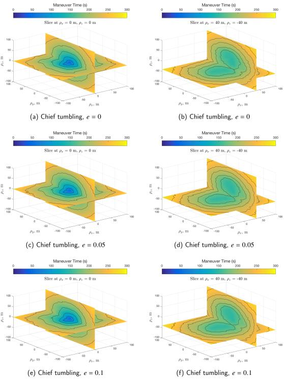
Figure 6.28. Comparison of relative position closed-loop backward T-reachable sets for chief orbital eccentricities of e=0, e=0.05, and e=0.1.
