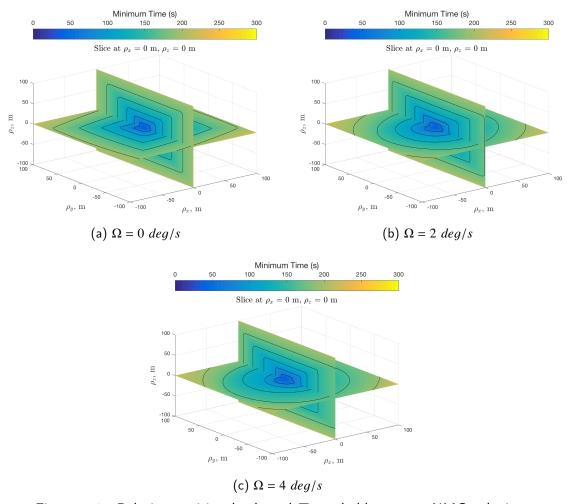
Figure 5.1. Relative position backward T-reachable sets at NMC velocity, aligned attitude, and zero angular velocity at different chief rotation rates, sliced at  $\rho_x = 0$  m and  $\rho_z = 0$  m; color bar indicates minimum time values corresponding to the contours.
