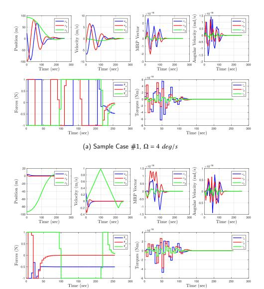
Figure 6.7. Sample NMPC closed-loop cases from position (NMC velocity, aligned attitude) for  $\Omega=4~deg/s$ .
