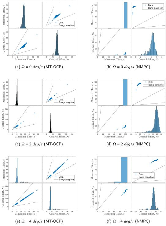
Figure 6.10. NMPC maneuver time and control effort histograms and correlation for attitude (zero angular velocity, rendezvous position) subspace.
