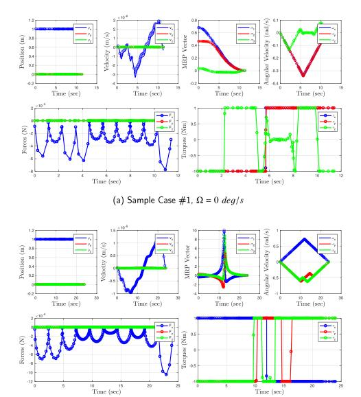
Figure 5.10. Sample cases from attitude (zero angular velocity, rendezvous position) subspace for  $\Omega = 0$  deg/s.
