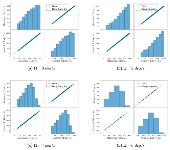
Figure 4.23. Minimum time and control effort histograms and correlation for velocity (R-bar position) subspace.
