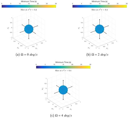
Figure 5.7. Relative attitude backward T-reachable sets at zero angular velocity and rendezvous relative position and velocity at different chief rotation rates, sliced at  $\sigma^T \sigma = 0.4$ ; color bar indicates minimum time values corresponding to the contours.
