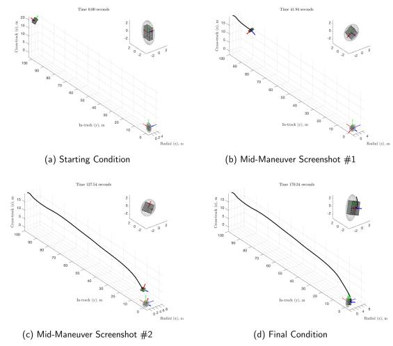
Figure 7.35. Case 5-relative trajectory for minimum time maneuver.
