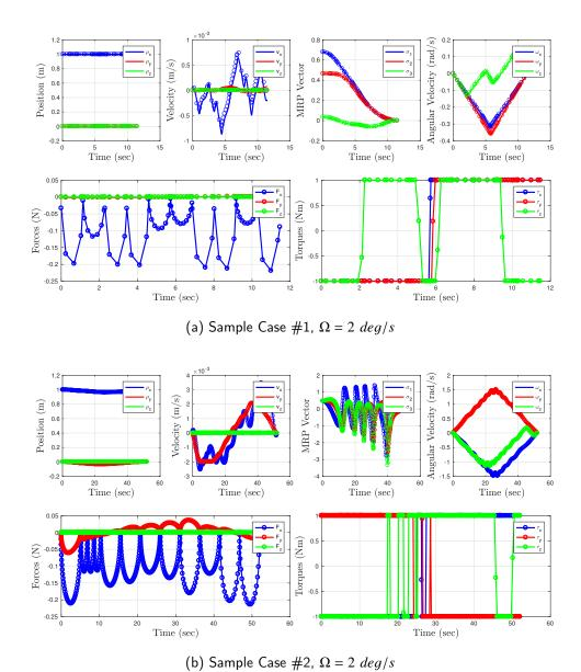
Figure 5.11. Sample cases from attitude (zero angular velocity, rendezvous position) subspace for  $\Omega = 2 \ deg/s$ .
