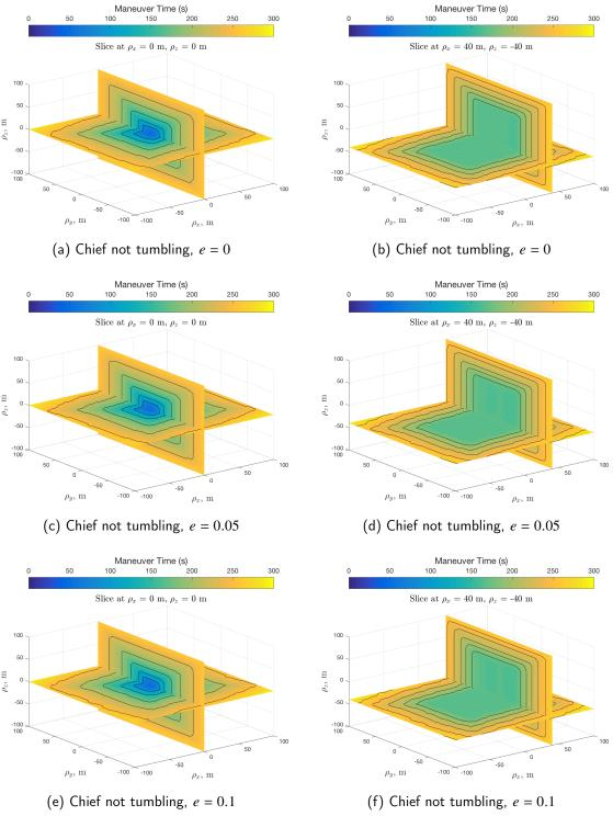
Figure 6.27. Comparison of relative position closed-loop backward T-reachable sets for chief orbital eccentricities of e=0, e=0.05, and e=0.1.
