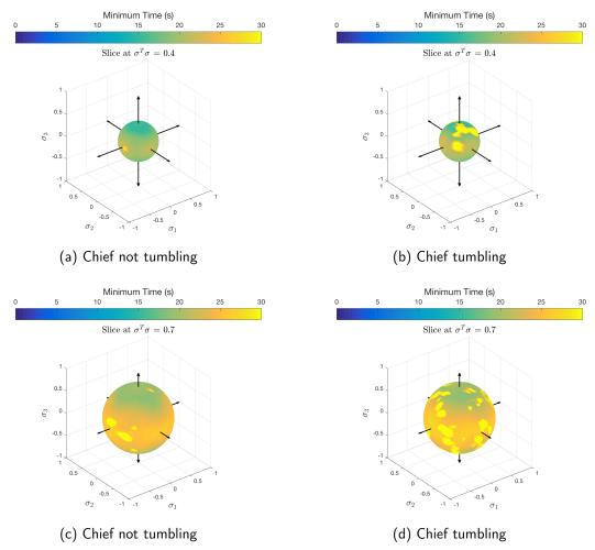
Figure 5.17. Relative attitude backward T-reachable sets at zero angular velocity and rendezvous relative position and velocity with tumbling chief, sliced at  $\sigma^T \sigma = 0.4$  and  $\sigma^T \sigma = 0.7$ ; color bar indicates minimum time values corresponding to the contours.
