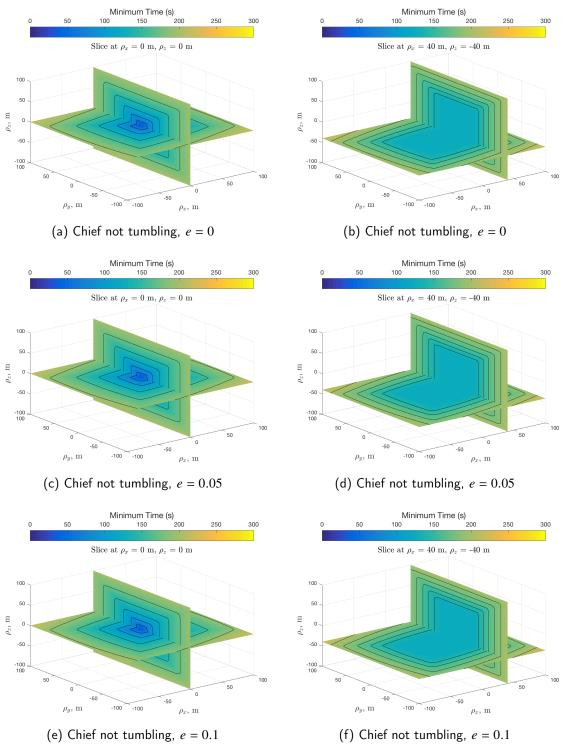
Figure 5.21. Comparison of relative position backward T-reachable sets for chief orbital eccentricities of  $e=0,\ e=0.05,\ {\rm and}\ e=0.1.$
