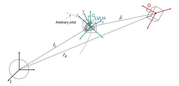
Figure 4.1. Depiction of general setup for the problem of rendezvous with a tumbling object.
