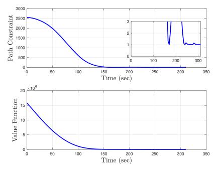
Figure 7.34. Case 4–verification of KOZ constraint satisfaction and time history of NMPC value function.
