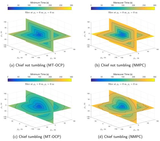
Figure 6.15. Relative position closed-loop backward T-reachable sets compared to traditional backward T-reachable sets.
