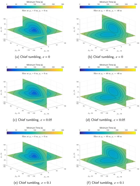
Figure 5.22. Comparison of relative position backward T-reachable sets for chief orbital eccentricities of e=0, e=0.05, and e=0.1.
