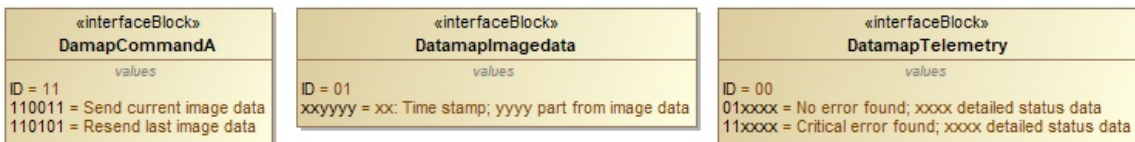
Figure 15. Modeling of Transport Layer Aspects as Proxy Ports for Leveraging Model Complexity (Salado & Wach, 2019)
