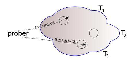
Yarrp iterates through randomly permuted < Target, TTL > pairs
