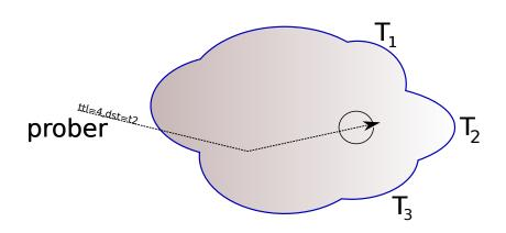
Yarrp iterates through randomly permuted < Target, TTL > pairs
