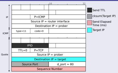
ICMP TTL exceeded replies permit recovery of: target probed, originating TTL (hop), and responding router interface at that hop.
