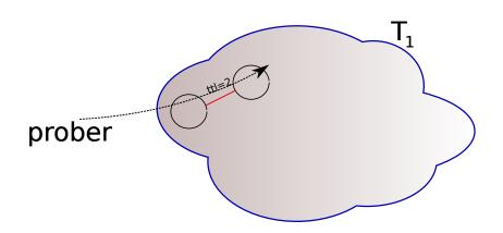
Traditional traceroute sends probes with incrementing TTL to destination  $T_1$
