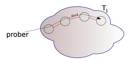
... continuing until finished with  $T_1$  (reach destination or gap limit). Prober must maintain state, while traffic is concentrated on *prober*  $\rightsquigarrow T_1$  path
