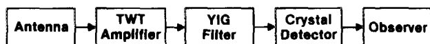
FIG. 2. Block diagram of the microwave antenna-detector apparatus. Horn antennas were used to observe frequencies above 8 GHz and a pyramidal antenna was used to observe below 8 GHz. Crystal detectors and TWT amplifiers were matched to the frequency sensitivity of the antennas. The YIG filter was tunable from 1–18 GHz. A frequency resolution of \pm 20 MHz was attained in these measurements.
