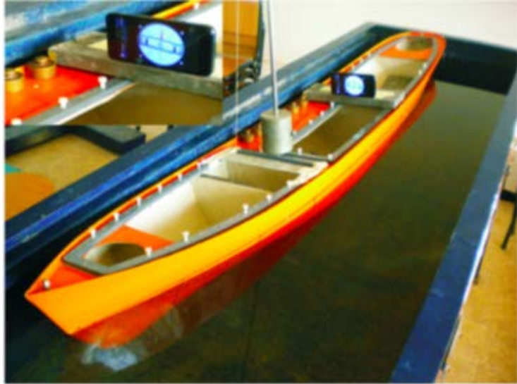
Figure 7. Experimental Set-up of BRSA Trawler for the Experiment. Source: Djebli et al. (2015).
