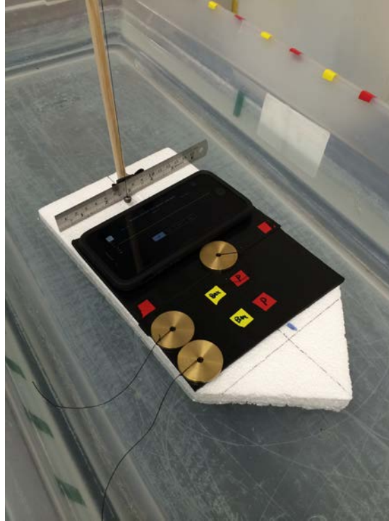
Figure 25. Picture of the V-Hull Model with Two Test Weights Shifted to the Starboard Side.
