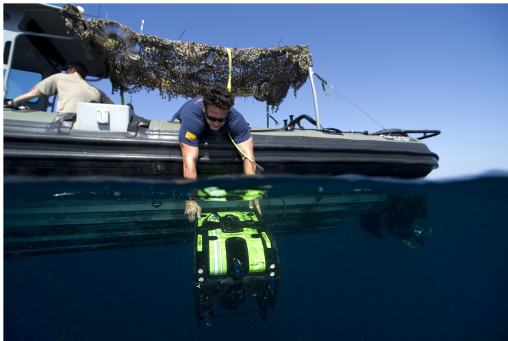
Figure 1.2. A Sailor launches a SeaBotix ROV from a small boat. Source: [3].
