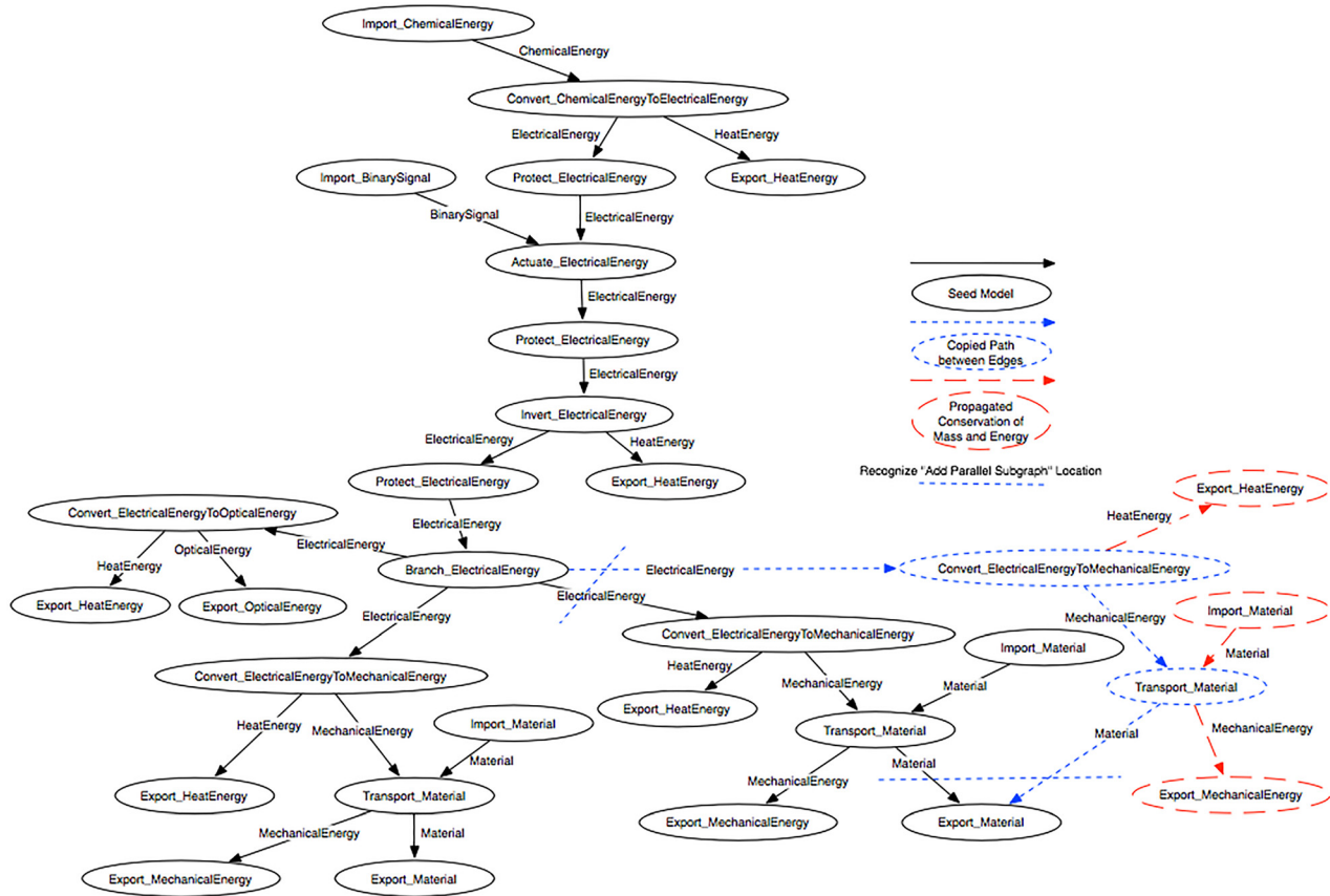
Fig. 3 Functional model of electrical power system
