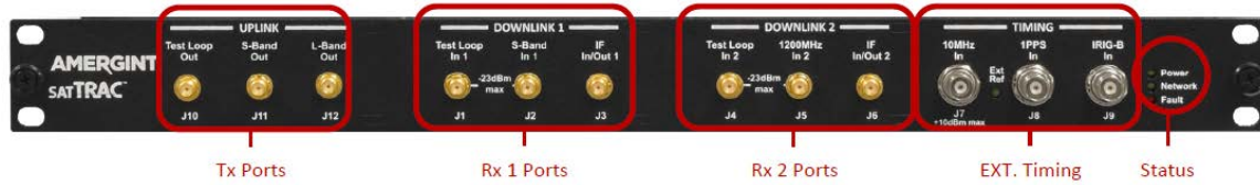
Figure 23. Annotated picture of the satTRAC Signal Converter front plate of RUS-4. Source: [22].
