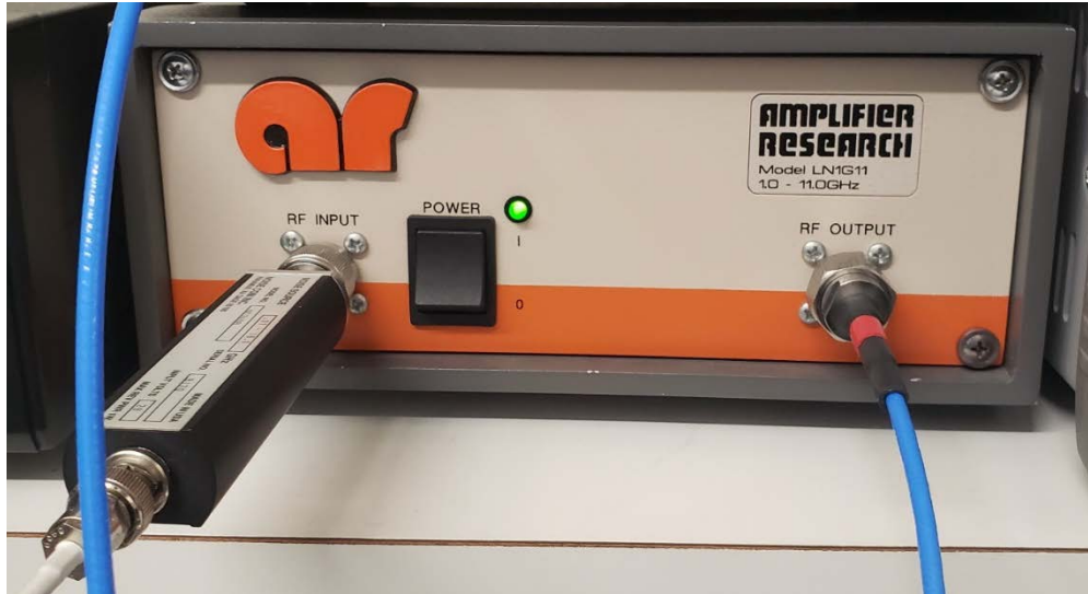
Figure 31. LN1G11 preamplifier used during noise figure measurements with HP 346B noise source attached.
