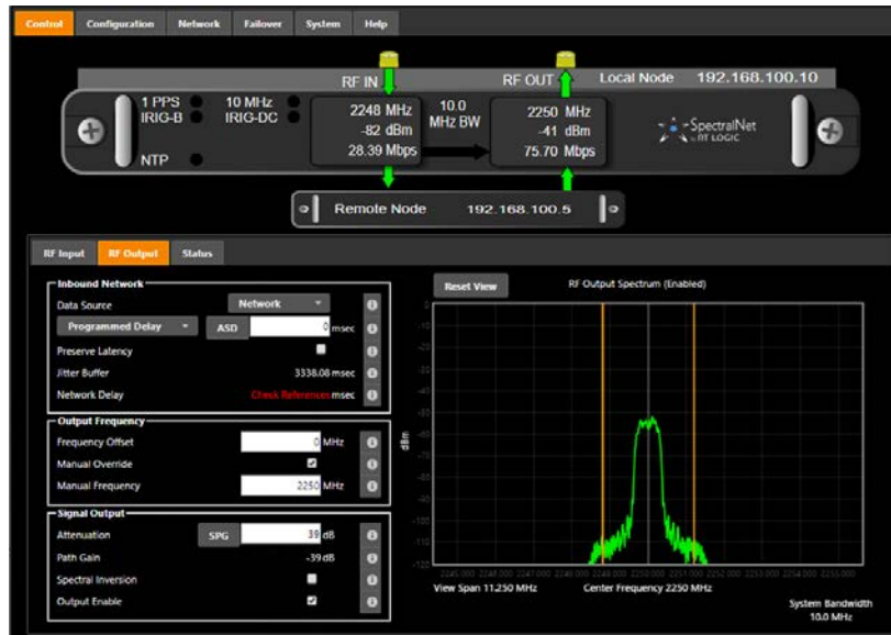
Figure 47. SpectralNet GUI programmed to transmit the standard test signal used during experimentation.
