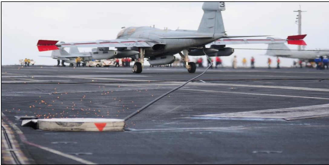
Figure 4. An EA-6B Prowler, Assigned to the “Rooks” of Electronic Warfare Squadron One Three Seven (VAQ-137), Catches One of Four Arresting Wires on the Flight Deck of the Aircraft Carrier USS Enterprise (CVN 65). Source: Pogo (n.d.).
