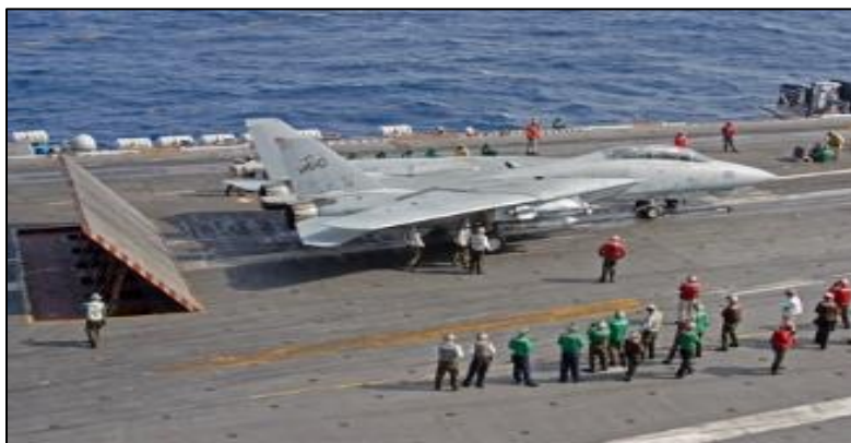
Figure 3. An F-14 Tomcat Preparing for Launch with the JBDs in Position to Deflect the Exhaust. Source: Avikerensky (2011).
