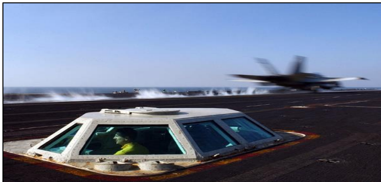
Figure 2. Aircraft Shooters Watch from Inside the ICCS Source: United States Navy (n.d.).
