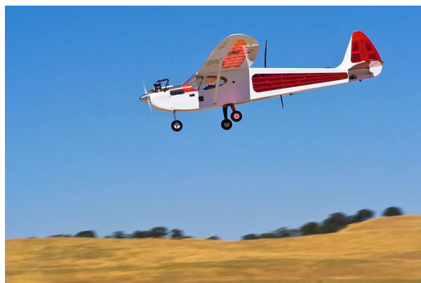
Figure 4: SIG Rascal 110 research aircraft operated by the Naval Postgraduate School for time-critical cooperative missions. Onboard avionics include the Piccolo Plus autopilot, two PC-104 industrial embedded computers, and a wireless MANET link for air-to-air and air-to-ground communications.
