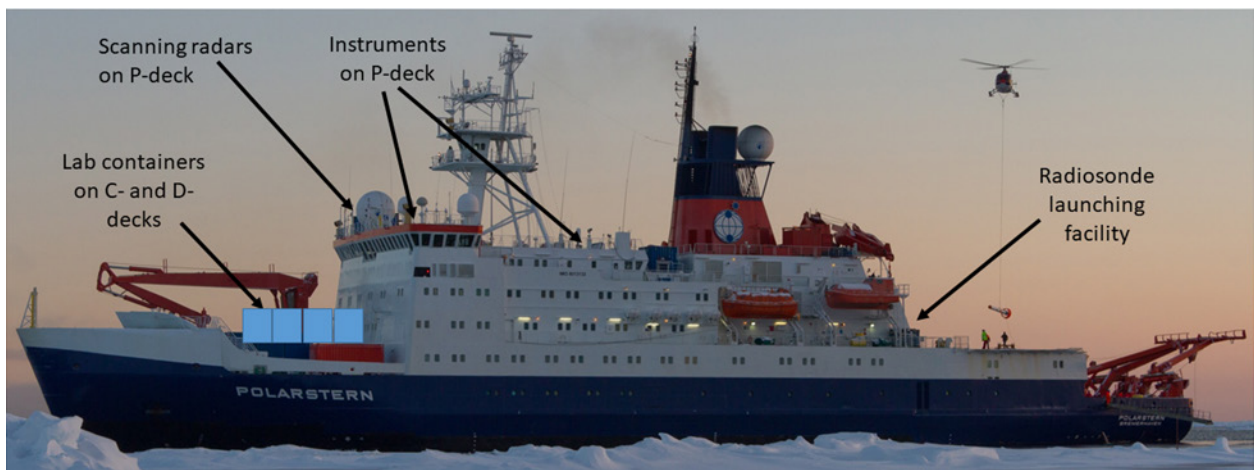
Figure 8. Polarstern with annotations designating installation locations for ARM Facility equipment.
