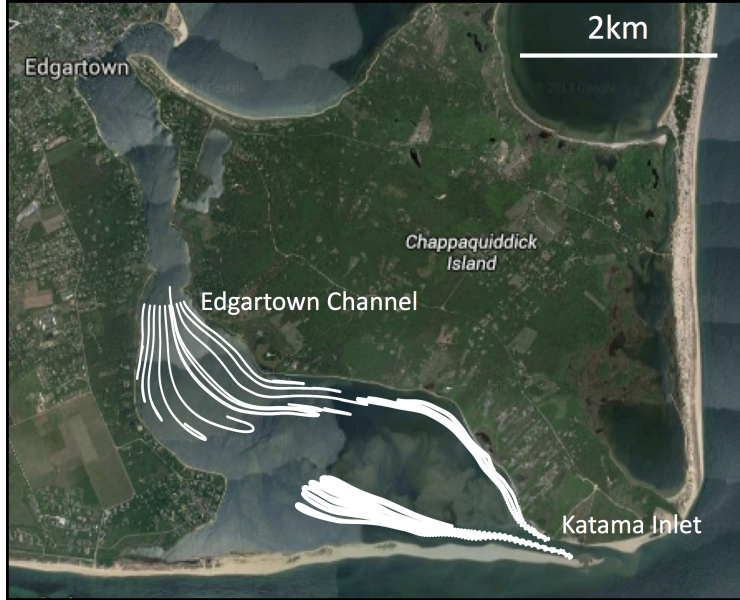
Figure 4: Synthetic drifter trajectories in Katama Bay. Thin white trajectories are from the drifters released on model date Aug 20 in Edgartown Channel, and thick white trajectories are from drifters released on model date Aug 22 just outside Katama Inlet.
