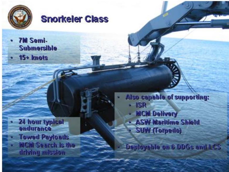
Figure 4. Snorkeler Class USV. Source: Department of the Navy (2007).
