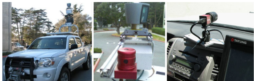
Fig. 2 Our vehicle setup. The Velodyne LiDAR is visible on top and a PtGrey Ladybug panoramic camera in front. The forward-looking camera is mounted on the dashboard next to a touchscreen display for visual feedback
