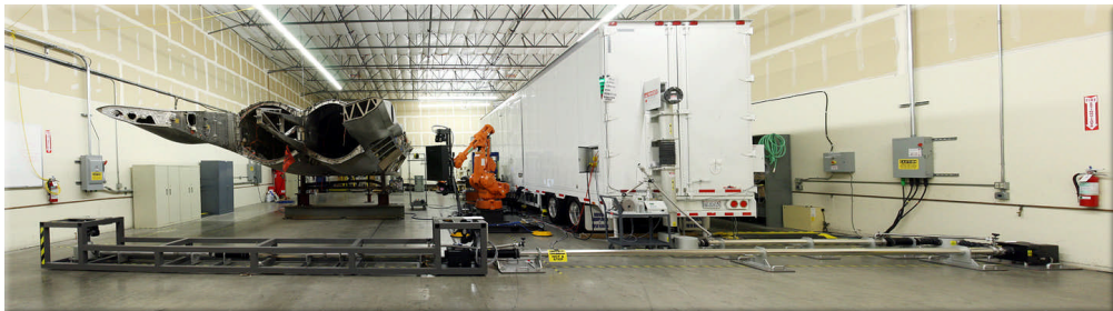
Figure 7 – A transportable laser-peening system located has now been located in Palmdale, CA to support F-22 overhauls. Production setup for processing F-22 wing attachment lugs. Spot placement is adjusted to 0.1 mm accuracy on each laser shot.
