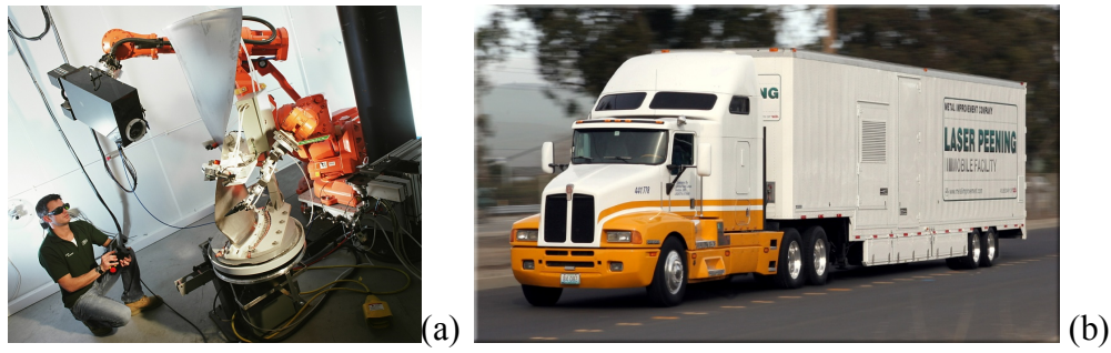
Figure 6– (a) The beam delivery robot during laser peening of a fan blade from a jet engine, and (b) one of four transportable systems now in operation. Laser Peening (LP) has been used successfully for stress mitigation in gas and steam turbine blades, the airframe of F-22 fighter jets, and arrestment hook shanks for aircraft carriers.
