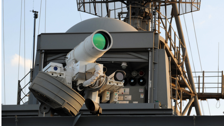
FIGURE 2.1 Picture of the U.S. Navy Laser Weapons System (LaWS) onboard the USS Ponce. Source: [12].
