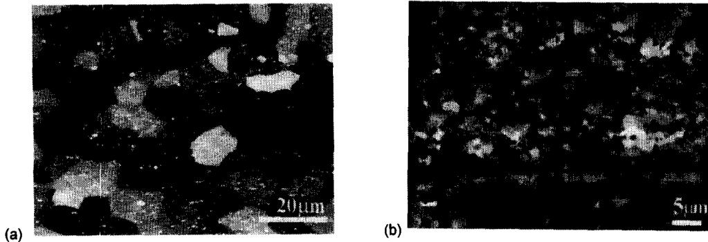
Figure 1. BSE micrographs of processed and annealed microstructures present in (a) SKY 5083 and (b) TMP6 Al-10Mg-0.1Zr. The rolling direction is horizontal. Orientation contrast, no etchant.
