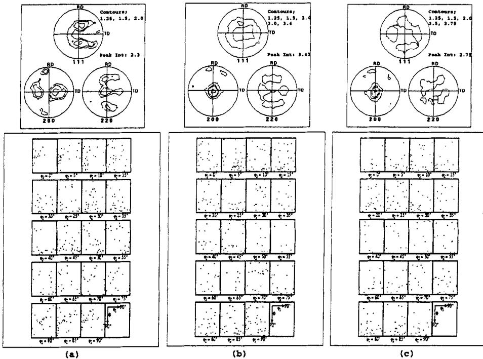
Figure 2. Microtextural plots for (a) as-received, (b) processed and annealed and (c) deformed specimens of SKY 5083.
