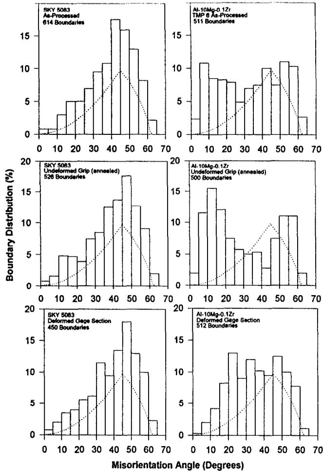
Figure 4. Grain misorientation histograms for specimens examined. The dotted line indicates the *continuous* plot of the probability distribution of misorientations for randomly oriented cubes predicted by Mackenzie [5].
