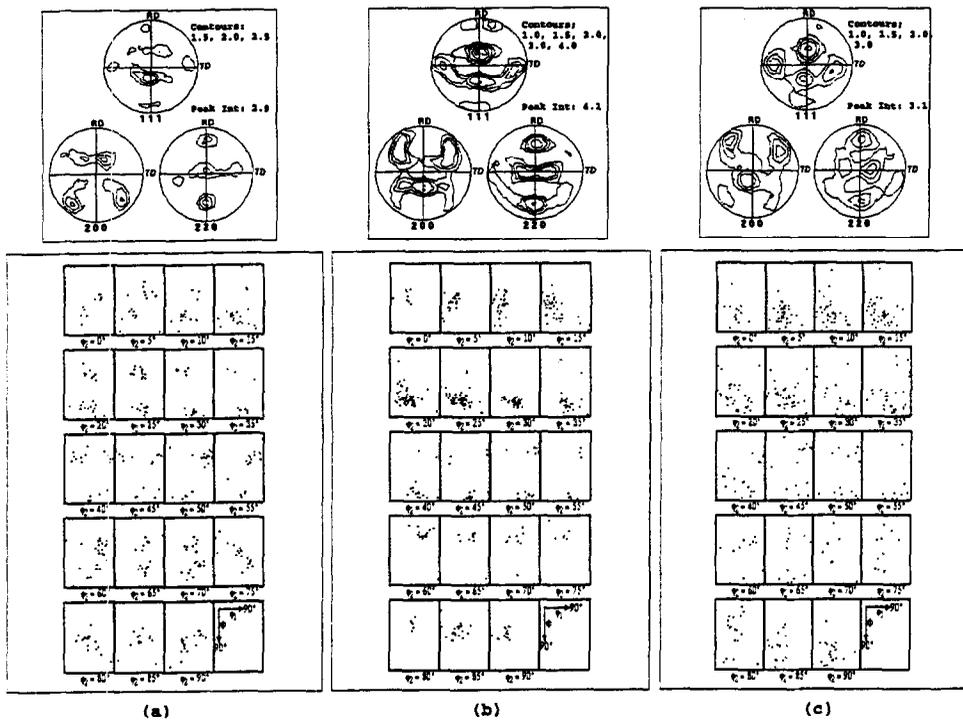
Figure 3. Microtextural plots for (a) as-processed, (b) processed and annealed, and (c) deformed specimens of TMP 6 Al-10Mg-0.1Zr.
