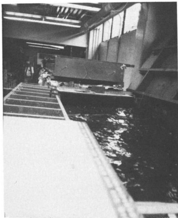
FIG. 1. Photo of OAWF from the end of the anechoic tank. The horizontal line in the middle of the photo is a breaker over the hydrophones.
