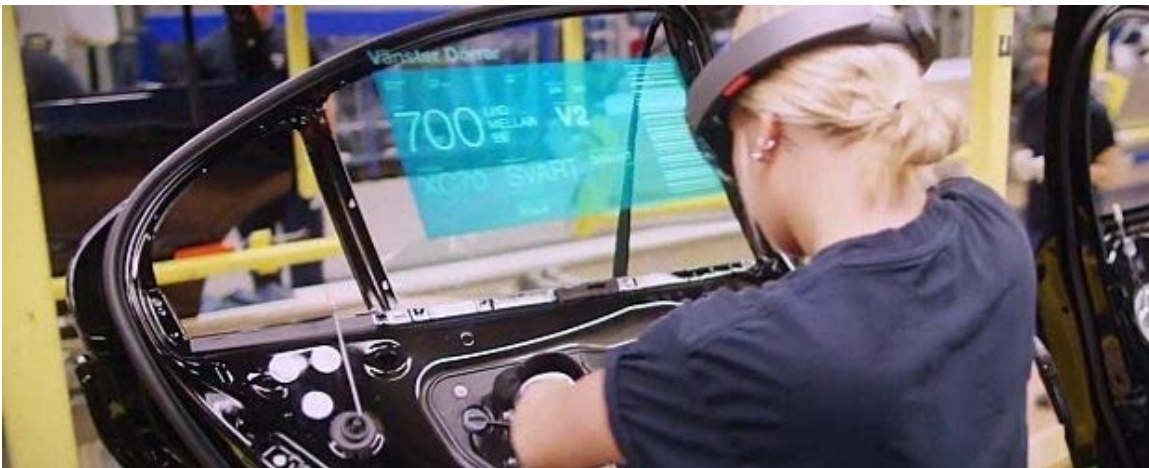
Figure 11. Volvo Using HoloLens for Assembly. Source: MacPhedran (2018).
