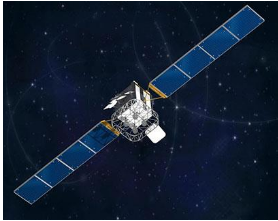
Figure 9. UFO Satellite Constellation Provides Tactical, Narrowband UHF Communications to the Navy and the DOD. 60
