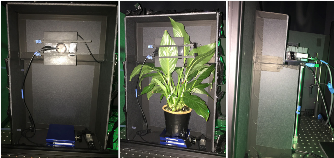
Figure 41. Plant test enclosure with front and sideview showing PMT
