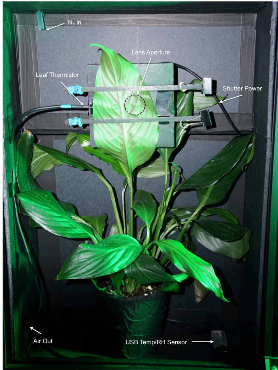
Spathiphyllum in plant enclosure (S). Shown with single filter lens assembly and front panel removed.
