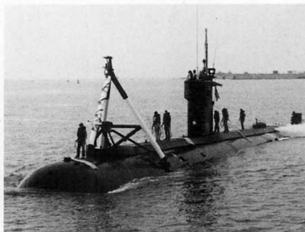
FIG. 1. The USS Dolphin (AGSS 555) with instrumentation mounted for the April 1982 measurements. Transducers for the turbulent velocity and temperature fluctuations are atop the tripod.
