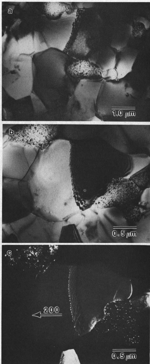
Fig. 5. Electron micrographs from the grip section of an elevated temperature test sample which has experienced approximately 3000 s total time at 573 K (300°C); (a) bright field showing fine grain structure with intergranular \beta precipitates; (b) bright field image showing a typical grain traversed by a subgrain boundary; (c) corresponding weak beam dark field (WBDF) image ( g/3g , B = [011] ) showing the spacing of dislocations comprising the subgrain boundary.
