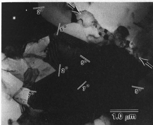
Fig. 7. Summary of the data from Fig. 6; misorientation angles, calculated from the orientation of neighboring grains relative to the reference grain (*), are shown. The range of values is similar to that observed in material which has experienced shorter annealing times (Fig. 4).
