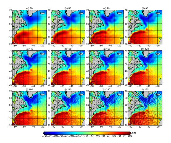
Figure 1: The mean dynamic topography (MDT) of the North Atlantic, based on the CLS01 mean sea surface and the 3rd generation GOCE time-wise gravity model, with truncations of the spherical harmonic expansion of the MDT ranging from L=30 to 250 in intervals of 20.
