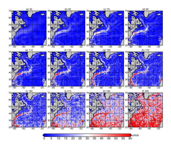
Figure 2: The mean geostrophic surface current speeds of the North Atlantic, obtained from the MDTs shown in Fig. 1
