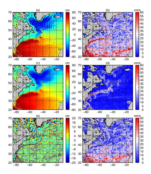
Figure 4: (a,b) The GOCE MDT for L=220, and associated geostrophic surface current speed field. (c,d) The optimally filtered GOCE MDT for L=220, and associated current field. (e,f) The difference between the filtered and unfiltered fields, i.e. what the filter removes.
