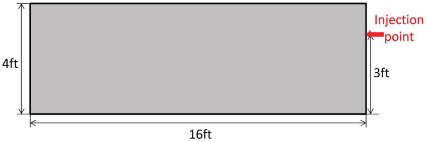
Figure 4.13. Demonstration of the 2D model for proppant transport verification
