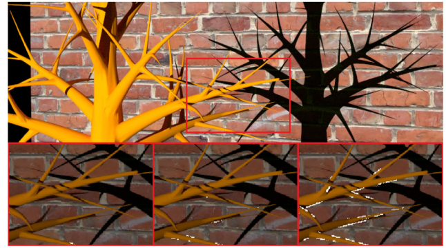
Figure 7: Detected shadow silhouettes (marked in white) on a mesh with \sim 183k triangles at 1, 10 and 100 importance iterations. While not all silhouette triangles are found, the remapping of importance from a lower resolution mesh increases the effective number of silhouette triangles found.
