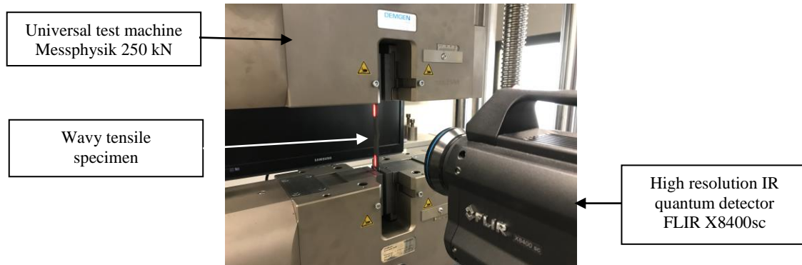
Figure 2: Passive thermography test set-up for tensile test.
