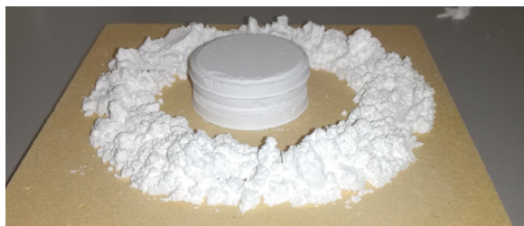
Fig. 2. Stacked disks surrounded by loose CaP1.0r powder for the second round of experiments in the closed furnace.
