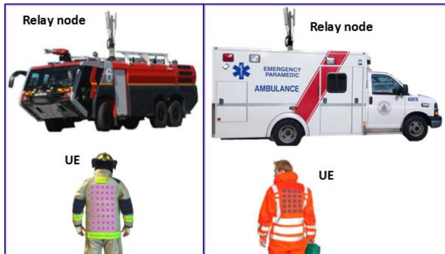
FIGURE 4.4: Example of temporary deployment for fire and medical brigades. Relay node mounted on the respective vehicles and textile antenna array deployed at the backside of the rescuers' jacket.
