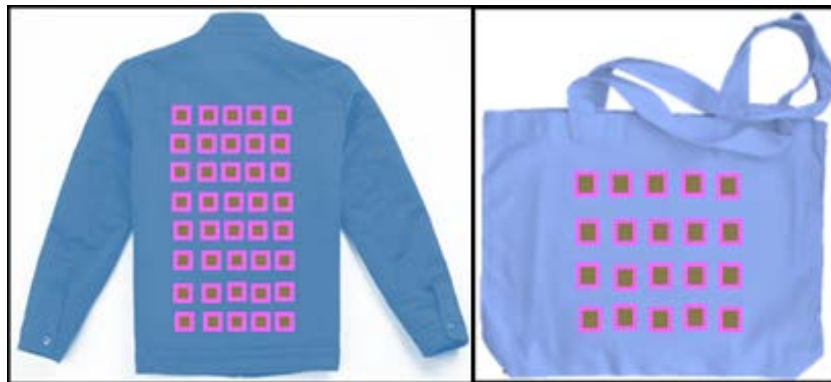
FIGURE 2.1: Textile multi-antenna deployed at user's garment. 8 \times 5 MIMO textile antenna array deployed at the backside of a jacket (left side) and 4 \times 4 textile antenna array deployed on a handbag (right side).
