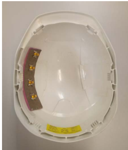
FIGURE 2.12: Experimental prototype of the conformal antenna inside a safety helmet.
