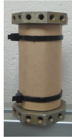
Fig. 1 Solid insulation test specimen
