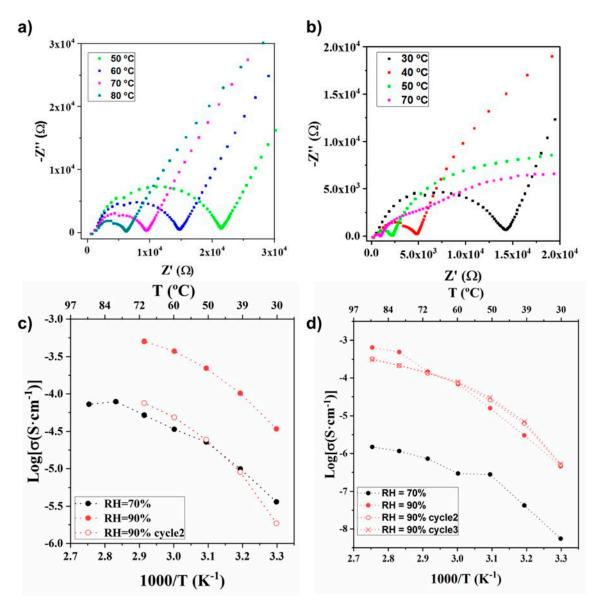
**Figure 3.** Nyquist plots for UPG-1 collected at 70% RH (**a**) and at 90% RH (**b**) and different temperatures. Arrhenius plots for UPG-1 (**c**) and Lys@UPG-1 (**d**), respectively, exhibiting the evolution of the proton conductivity vs. temperature at 70 and 90% RH. Recyclability of both UPG-1 and Lys@UPG-1 at 90% RH is also represented.
