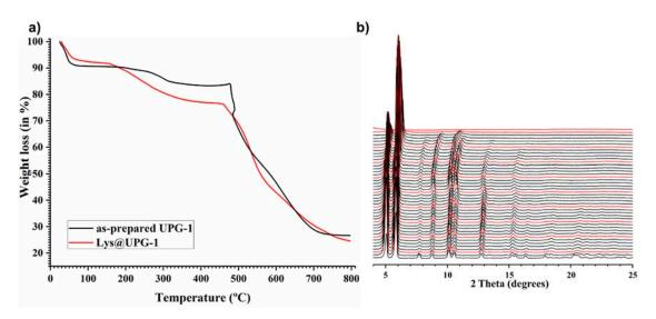
**Figure 2.** (a) Thermogravimetric analysis (TGA) of UPG-1 and Lys@UPG-1 and (b) VTPXRD patterns of UPG-1 from 30 to 500 °C. Each red line corresponds to an increment of 50 °C. No significant structural changes are observed up to ca. 440 °C, besides some shift of the peaks, at higher temperatures (i.e., from ca. 350 °C) and loss of crystallinity after ca. 400 °C. An amorphous residue appears at about 500 °C.
