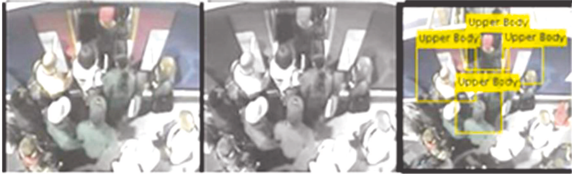
Figure 7. Cascade or Viola-Jones [41, 43] algorithm for upper body passenger detection: (a) red, green and blue frame; (b) preprocessed frame; (c) final passenger detection.
