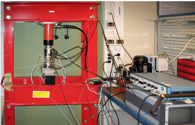
Figure 6. The ultrasonic uniaxial rock measurement setup. A hydraulic cylinder is fixed to the top of the steel frame inside which the transducer-sample assembly resides. A load cell- and thermocouple-amplifiers are placed on the right side of the frame. The hydraulic motor and relay control unit are behind the oscilloscope and pulser/receiver. The PC and the optional cooler and oven are outside the picture.
