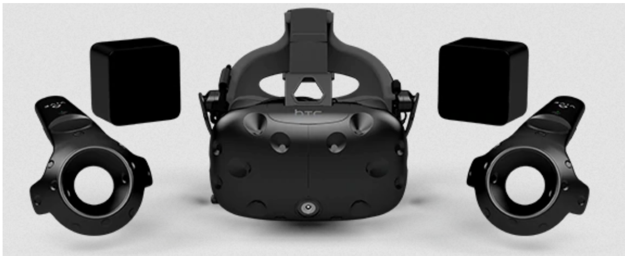
Figure 1.1: The HTC Vive virtual reality set used in this work [11]. The set contains a head-mounted display (HMD), two base stations and two wand controllers.
