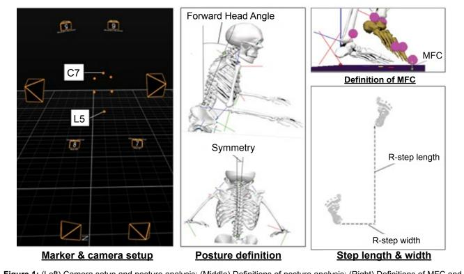
Figure 1: (Left) Camera setup and posture analysis; (Middle) Definitions of posture analysis; (Right) Definitions of MFC and step length & width.
