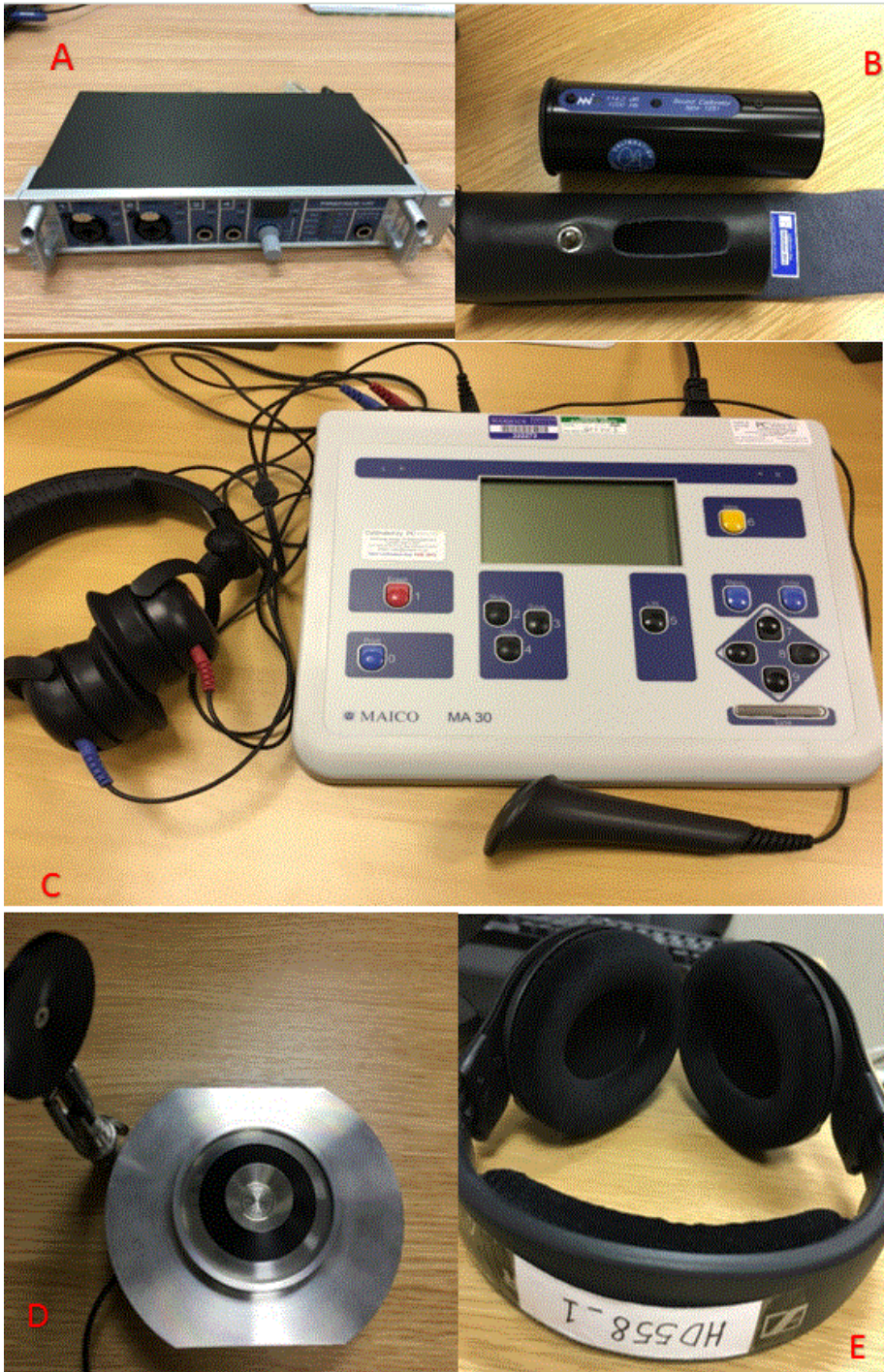
Fig. 3.4 Pictures of the apparatus used in the experiments: A, Sound Amplifier; B, Sound Calibrator; C, MAICO30 Clinical Audiometer; D, IEC 711 coupler; E, Headphones
